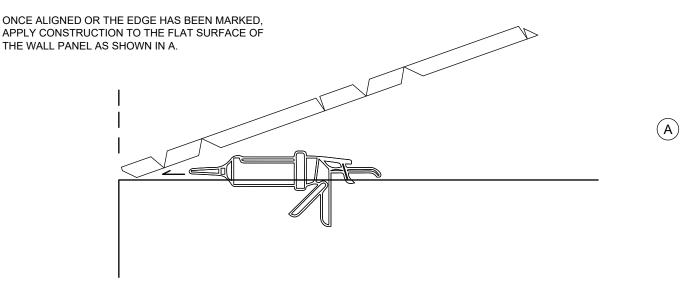
NOTE: ADHESIVE SHOULD ONLY BE APPLIED TO PART HIGHLIGHTED BELOW
